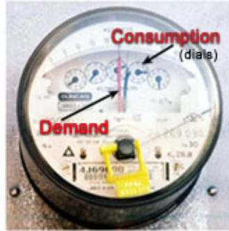
Commercial Electric Meter
