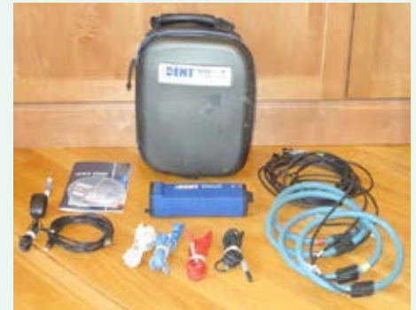
Dent Instruments ELITEpro XC with voltage cables, available current transducers and carrying case.
